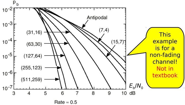
Drawbacks with long codes is complexity and delay.
