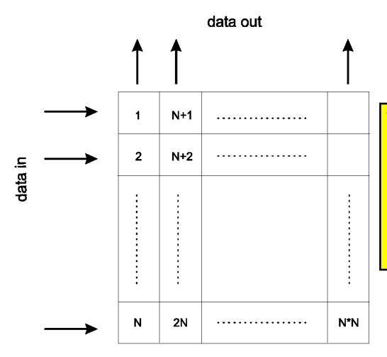
The writing and reading of data in interleavers cause a delay in the system, which may cause other problems.
