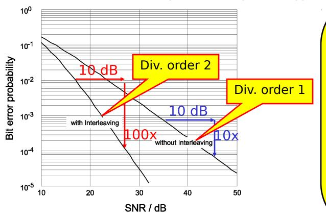
Hard decoding of block codes with minimum distance  $d_{min}$  gives a code diversity order of d = -1
