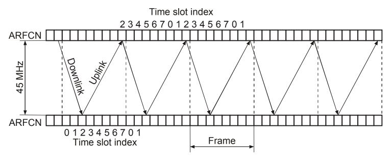
The MS transmits to the BS three time-slots after it receives a transmission from the BS.
