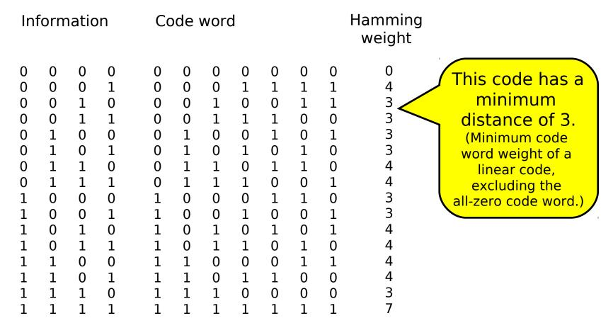
This is a (7,4) Hamming code, capable of correcting one bit error.
