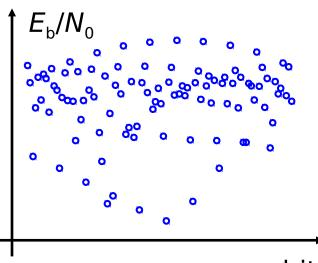
bit With interleaving the fading dip spreads more evenly across code words
