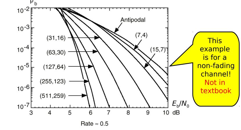
Drawbacks with long codes is complexity and delay.
