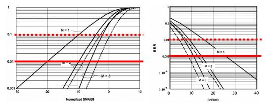
a) Inspecting the outage figure (left – solid horizontal line) we see that 1% outage is reached at fading margins (how far down is the 1% level) 21 dB for 1 antenna, 10 dB (RSSI) or 8 dB (MRC) for 2 antennas, and 7 dB (RSSI) or 4 dB (MRC) for 3 antennas. This constitutes diversity gains (difference compared to only one antenna) of 11 dB (RSSI) or 13 dB (MRC) for two antennas
