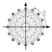
Calculating the "average ampliude" is not possible, unless we know the speed at which the linear transitions take place. It is, however, possible to find the dynamic range, namely the ratio between the largest and smallest amplitude (on the complex envelope). By assuming that the constellation points (max amplitude) are at radius 1, the **minimal amplitude** becomes  $\sin(11.25^\circ) \approx 0.195$ .
