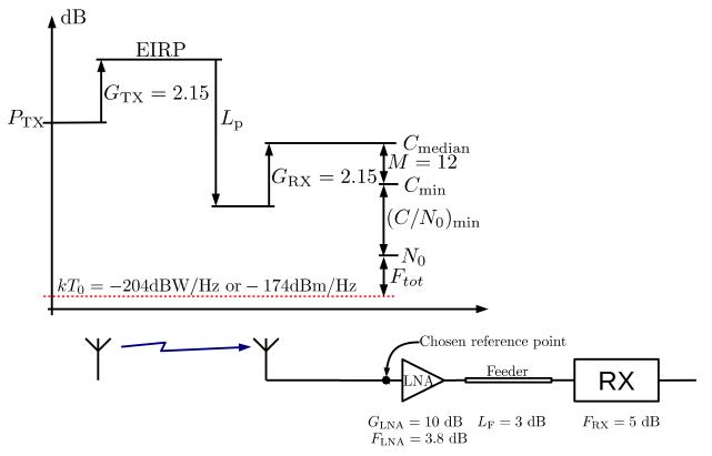
Several of the variables in the link budget are not yet calculated. Let's start with the propagation loss  $L_p$ . Since propagation takes place in a *large city* (metropolitan area) and all parameters fall within the valid ranges, we choose the Okumura propagation model.
