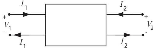
Figure 3.1: A two-port. Notice that the total current entering each port is always zero.
