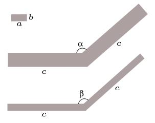
The figure shows two waveguides that each consists of two sections. The dimensions of the waveguides are a=10 cm, b=4 cm and c=50 cm. They are used in the frequency span 2.3-2.8 GHz. The waves are entering at the left port and exit at the right. Only the  $TE_{10}$  mode is used.
