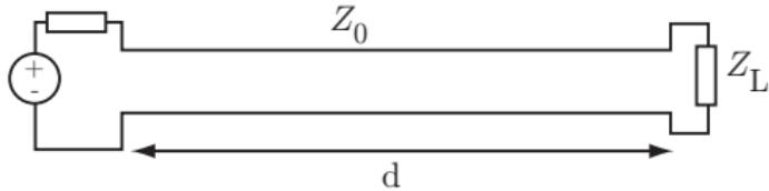
$$\Gamma(0) = \frac{Z(0) - Z_0}{Z(0) + Z_0} = \frac{Z_L - Z_0}{Z_L + Z_0} e^{-2j\beta d} = \Gamma_d e^{-2j\beta d}$$
