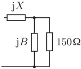
$$B = \frac{0.475}{50} = 9.5 \text{ mA/V} \text{ and } X = 1.38 \cdot 50 = 69 \text{ V/A.}$$
