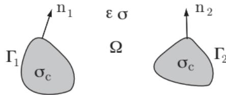
Solve Laplace equation  $\nabla^2 \Phi(x, y)$  in  $\Omega$ .
