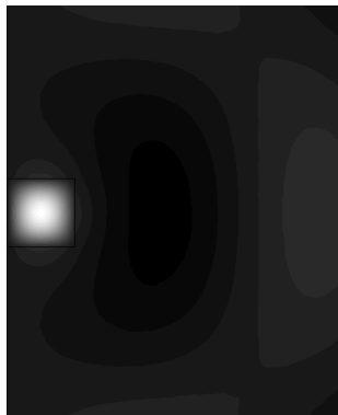
Figure 8.16: The magnetic field of the lowest resonant TM-mode. The frequency is f_r = 73.4 GHz for the cylindrical resonator with \epsilon = 10 , radius a = 1 mm and height h = 1 mm.
