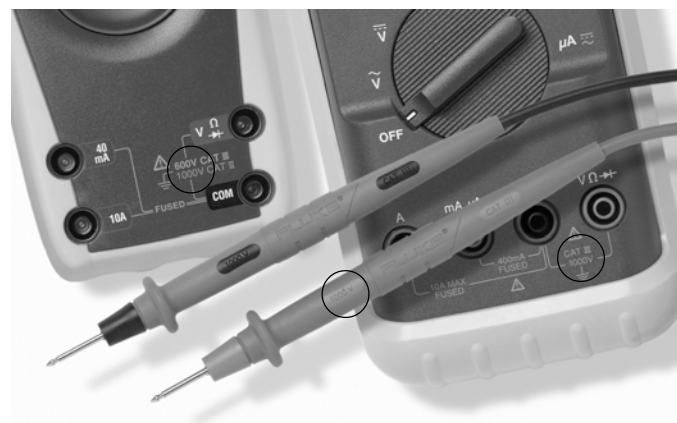
Look for category and voltage ratings of test leads and multimeters.
