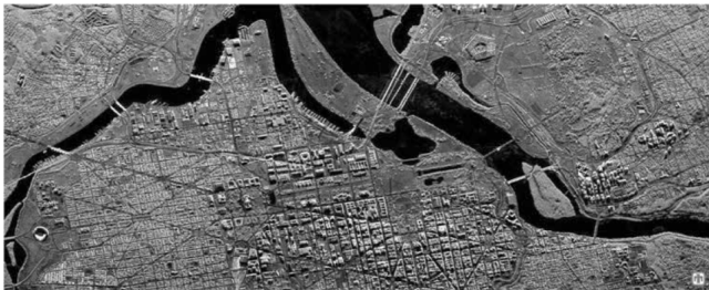
FIGURE 1-32 ■ 1 m resolution SAR image of the Washington, D.C., mall area. (Courtesy of Sandia National Laboratories. With permission.)
