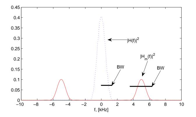
The carrier modulated signal is  $y_m(t) = y(t) \cos(2\pi t f_c)$ But bandwidth gets twice as large!
