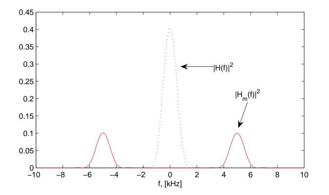
The carrier modulated signal is  $y_m(t) = y(t)\cos(2\pi t f_c)$
