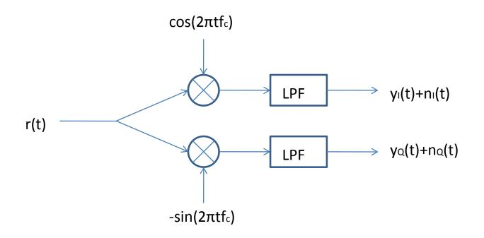
The in-phase and the quadrature components can be independently detected! The LPF (low pass filters) can be taken as a matched filter to h(t)
