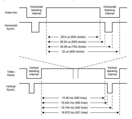
Figure 2: Signal timing diagram for a 60Hz, 640×480 VGA display.
