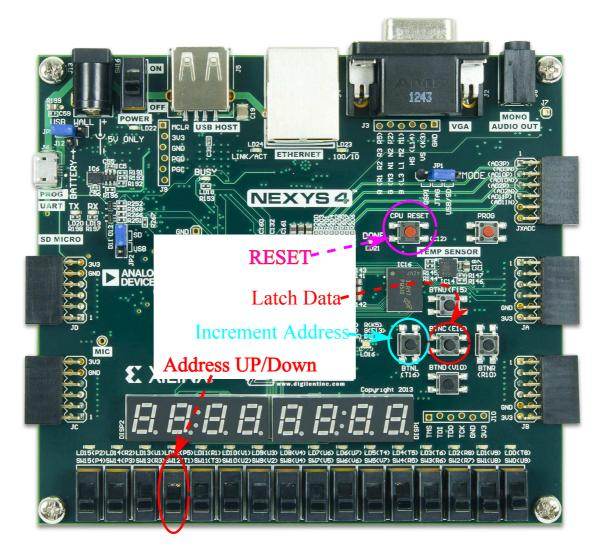
Figure 4: FPGA with memory controls
