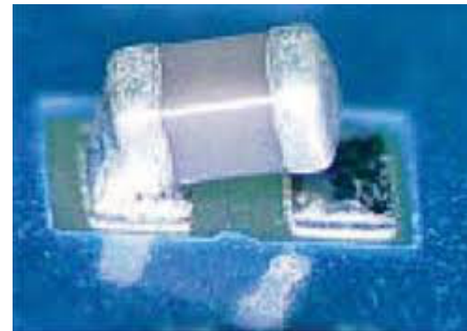
Fig. 1. With "tombstoning" only one side of a two-leaded chip component may be soldered to the target pad, but its other termination may not come in contact with the associated target pad. Photo courtesy of IPC-610
