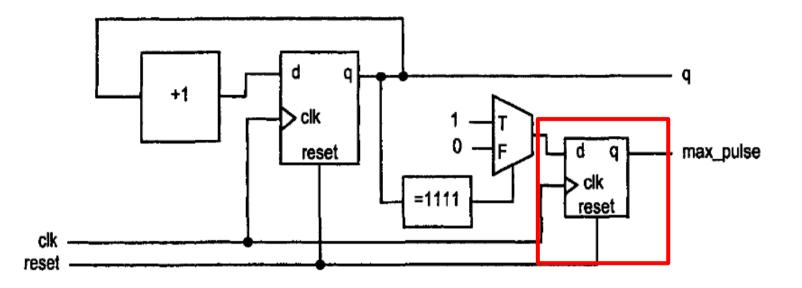
**A** 1-bit register is inferred for the max\_pulse signal.
