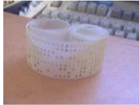
Punched paper tape, instruction stream in Harvard Mk 1 (1950s)
